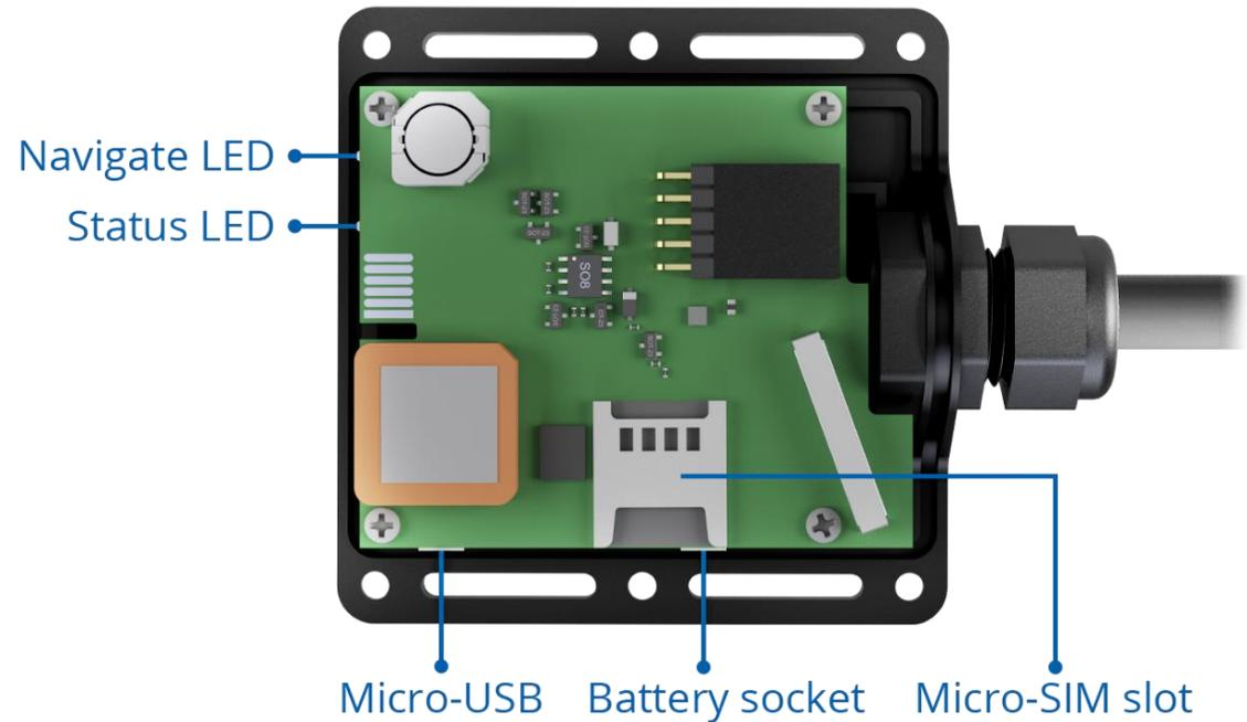
Figure 1 FMB209 device view
