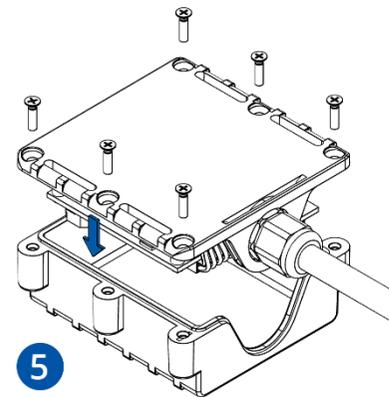
Figure 8 Attaching cover back
