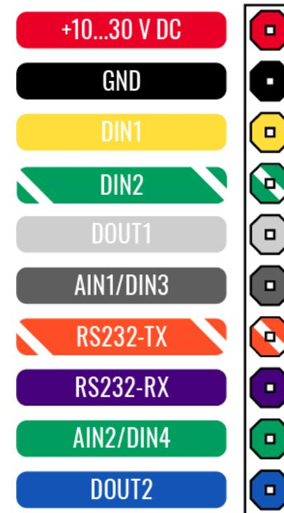
**Figure 2 FMB209 Pinout**
