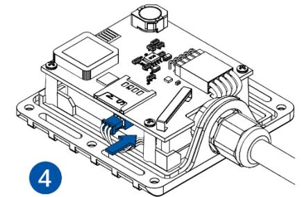
Figure 7 Battery connection
