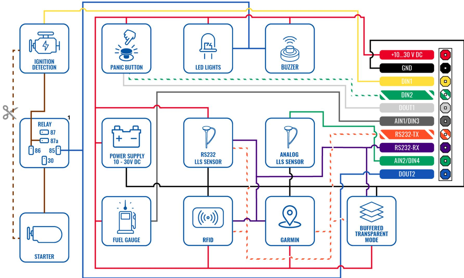
Figure 3 FMB209 Wiring scheme
