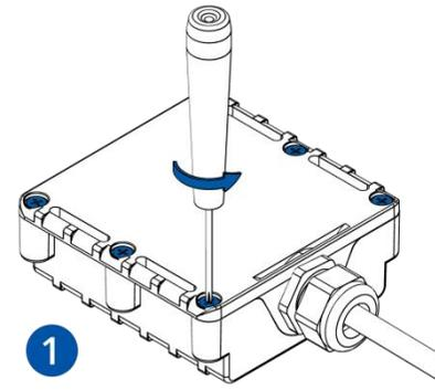
Figure 4 Unscrew screws
