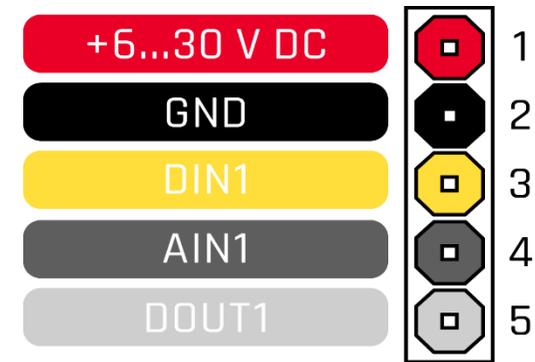
Figure 2 FMB910 pinout
