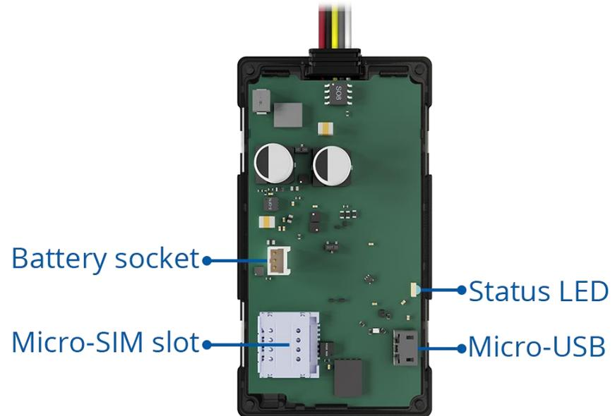
Figure 1 FMB910 device view
